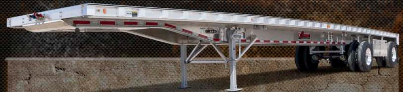
The Premier AF-1080 All Aluminum flatbed has a base weight of approximately 8,000 lbs. on a typical 48 ft. unit and a 23" main beam depth. The trailer features one-piece aluminum flanges and sections without any splices and its load capacity rating is among the highest in the industry.
