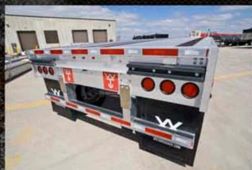
Roadbrute and Premier flatbeds are standard with an extruded aluminum rear end with aluminum R.I.G. (Steel R.I.G. is optional on the Roadbrute.)
