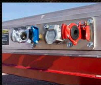
Wilson's redesigned front end has a cleaner, lower profile with gladhand and electrical hookups mounted on a removable access plate
