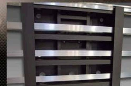
The **King Pin** area is coated inside and out with Corsol to seriously reduce corrosion in this critical area. The design is also void of any corrosion harboring tubes plus it makes use of the full-width aluminum crossbars which add strength while reducing the trailer's overall weight.
