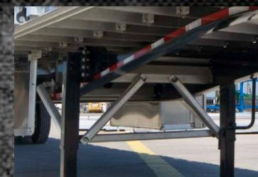
Aluminum landing gear braces are lighter than steel and withstand the beating from rocks and road debris.
