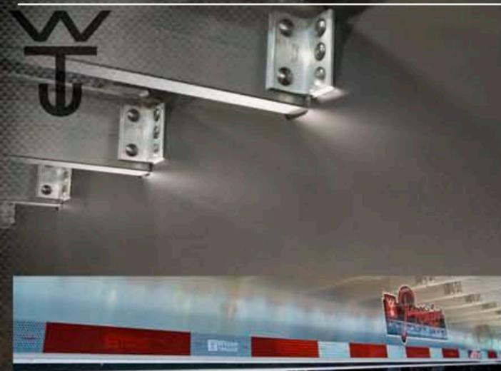
The main beams of the Roadbrute and Premier are manufactured with a crowned "mirror image" of each other. This precision cut camber or "arch" removes the possibility of high or low beams on a Wilson trailer.
