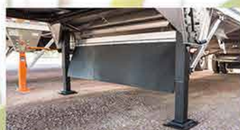
Full-width belting between landing gear legs
