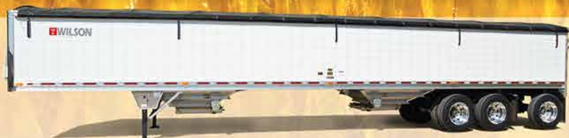
DWH-500 Pacesetter 50' long, 96" wide, 72" sides Dual-Dual-Single Non-Equalizing Rear Lift – 10'-2" Spread with 73" axle spacing between the center and rear axle.
