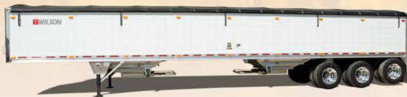
DWH-500 Pacesetter 50' long, 96" wide, sides 72" (Optional 2 rows of 9 lights) Dual-Dual-Dual Fully Equalizing Rear Lift – 9'-7" spread with two 57-1/2" axle spacings.
