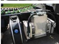
Junction boxes include wiring diagram labels inside. All utility boxes are manufactured from aluminum and all boxes are positioned for easy access.
